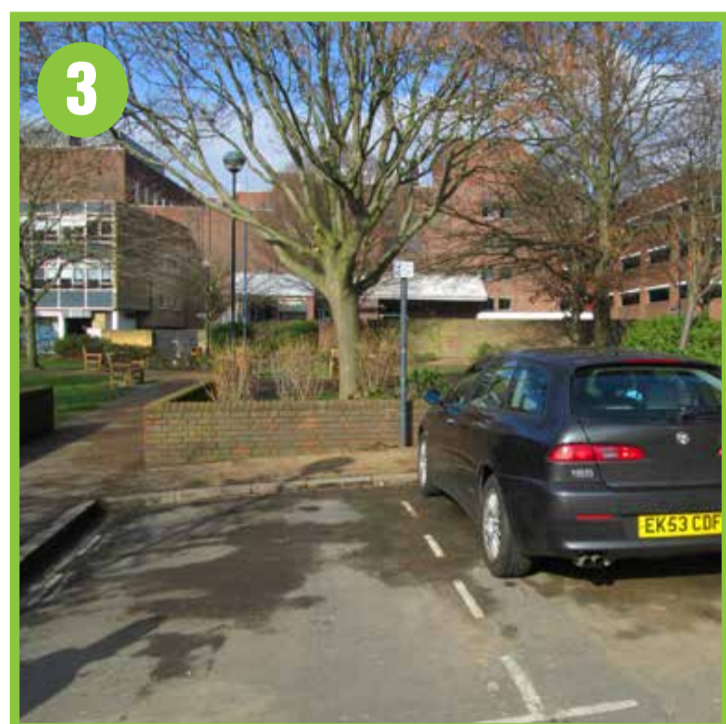
Remove parking in front of the park, at the end of Garfield Road. Reduce extents of retaining walls to increase the openness of the space and improve accessibility
